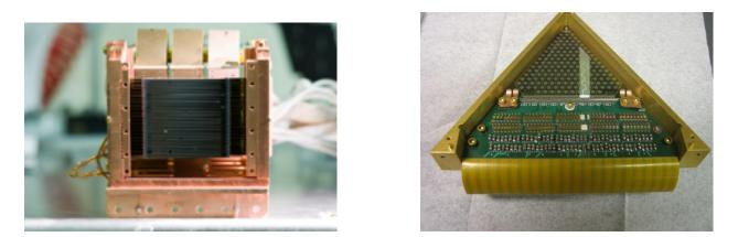
Figure 2: Detector arrays for ACT and SPT. On the left is one of the ACT arrays. It contains 32 by 32 detectors that were fabricated at NASA/GSFC. Cryogenic optics images the sky onto the 32 by 33 mm active area. Each strip of 32 detectors is built onto a silicon card. On the right is an image of a SPT sub array developed at Berkeley. The TES detectors are at the top. Feed horns (not shown) couple the radiation onto the detectors. The circuit board at the bottom contains multiplexing circuitry.
