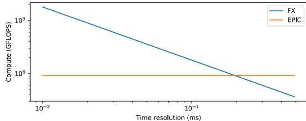
**Figure 3.** The computational cost for a hypothetical MWA-III with an EPIC-based (orange) and a correlator-based (blue) approach as the output cadence is varied. At faster cadence, the latter becomes less efficient.
