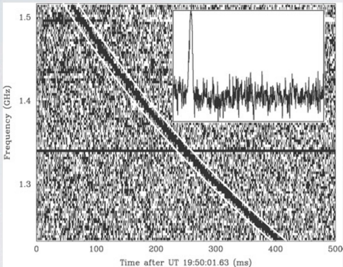
$$\Delta t_{\text{DM}} = 8.3 \mu\text{s DM} \Delta\nu_{\text{MHz}} \nu_{\text{GHz}}^{-3}$$
