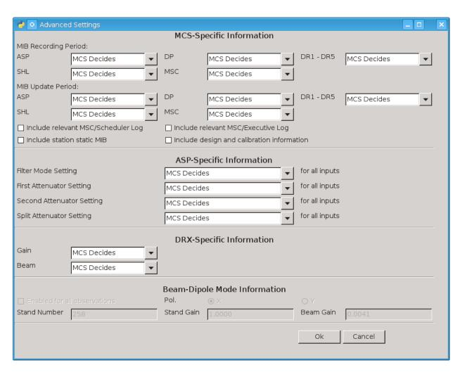
Figure 2: The sessionGUI.py advanced observation settings window. Here you can define the gain used for the observations and which beam DRX observations are to use.
