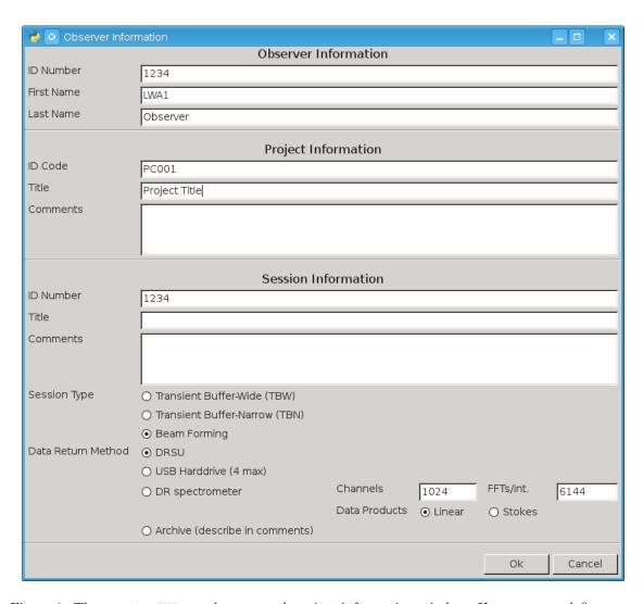
Figure 1: The sessionGUI.py observer and project information window. Here you can define your name, the project, the LWA1 mode to be used to collect the data, whether or not to use the data recorder spectrometer, and how the data are be to returned to you.
