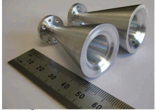
Smooth-walled spline feeds designed using analysis code based on mode matching along the horn length
