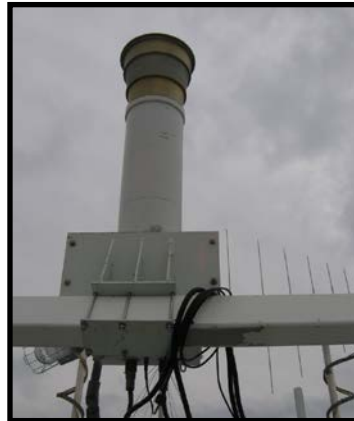
Reference receiver at top of feed arm
