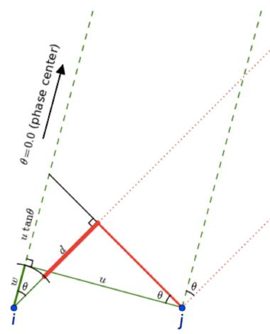
Consider direction-dependent arrival geometry for E-field disturbance reception at two points, i and j, relative to the phase center direction
