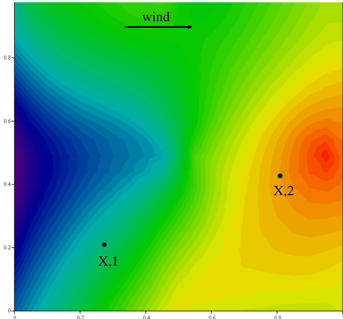
Target visibility sees the difference in delay between positions X,1 and X,2 in the phase screen which changes as the wind blows the frozen turbulence across the array.
