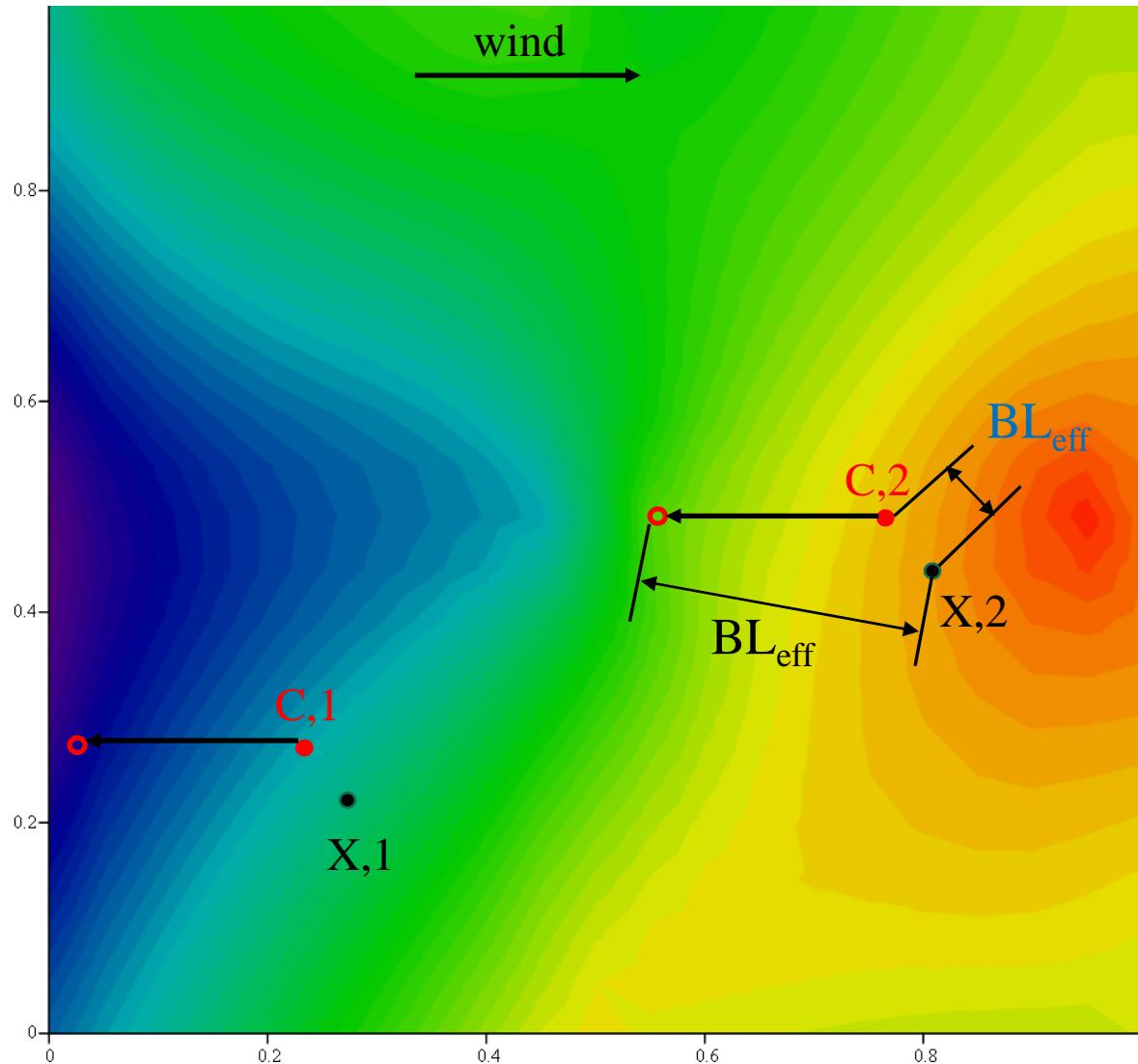
Under normal “slow” calibration the phase screen will have moved a significant distance during a target-calibrator cycle, greatly increasing  $BL_{eff}$
