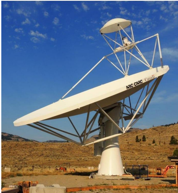
SKA Dish Verification Antenna 1 DVA-1 15 m
