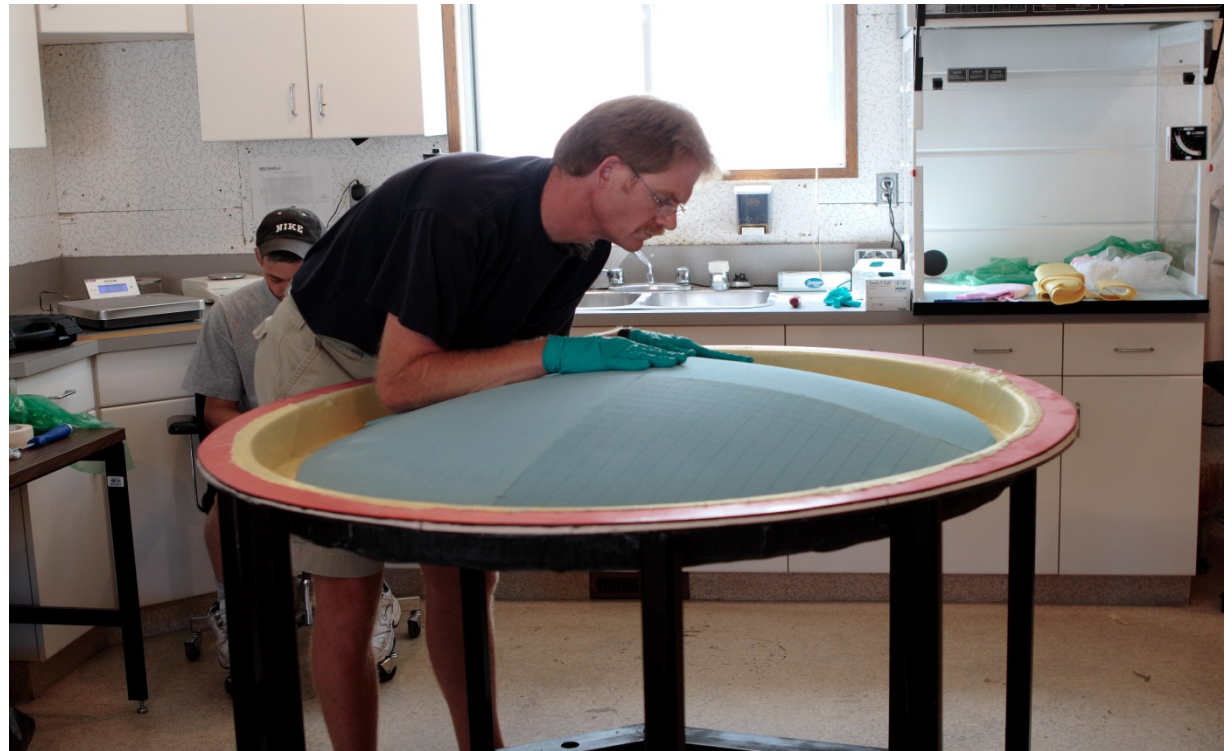
Laying up first 1 metre dish part.
