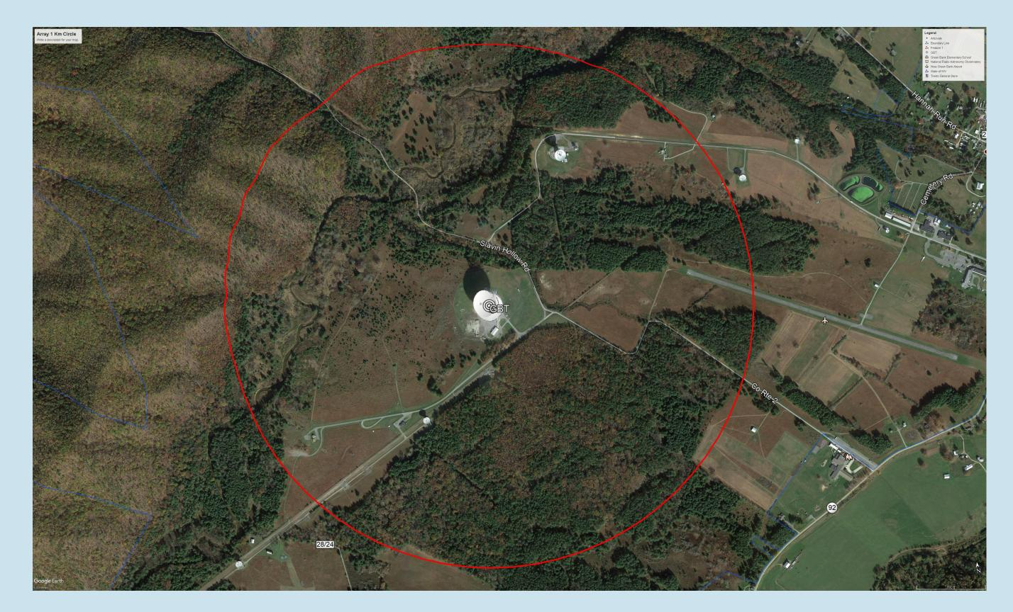
A 1 km radius around the GBT is shown above. The image is oriented such that north is up and east is right. Everything east of Deer Creek (roughly flowing from the upper center to the lower left corner of the image) is fairly level. Terrain west of Deer Creek is mountainous. Power and optical fiber is easily accessible east of Deer Creek.
