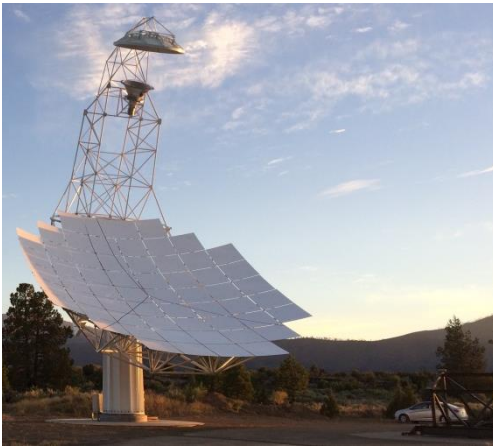
A glass antenna reflector made by thermoforming
