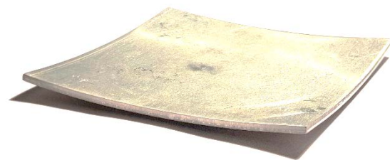
Figure 3. Slumped aluminum test plate example, having a lower focal length to show curvature.
