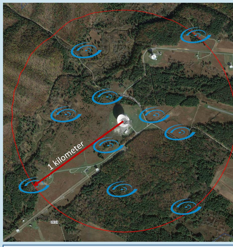
The Green Bank Array would lie within 1 kilometer of the Green Bank Telescope. Ten possible locations for ngVLA antennae are shown here, though we have not yet completed a detailed study of array location. Terrain north and west of the telescope is mountainous, while fiber and power are readily accessible elsewhere.
