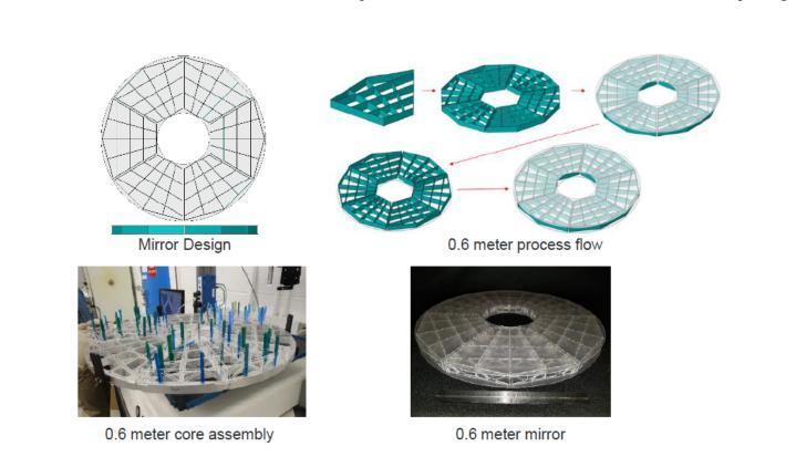
Constructed Core technology leverages commoditized core components with faceplate replication to provide rapid, affordable mirror solutions
