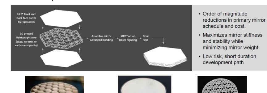
3D printing enables volume optimization of mirror cores for ultralightweight designs
