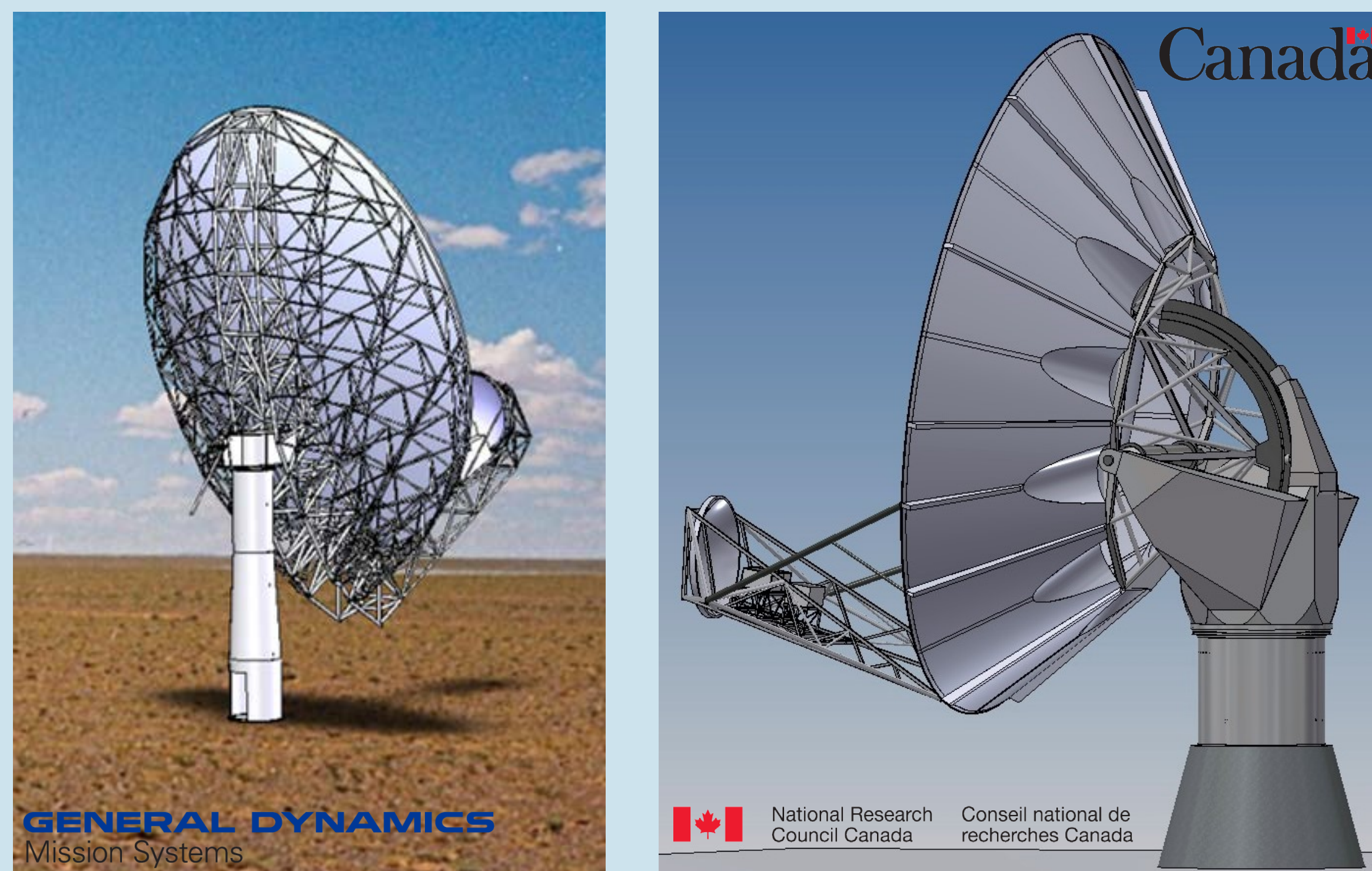
Figure 3: GDMS 18 m (Left) and NRCC 18m (Right) Antenna Concepts. Courtesy of GDMS and NRCC.
